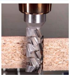
Diamaster PRO<sup>3</sup> (left) – the first choice for sizing on nesting machines and batch size 1 machines.
