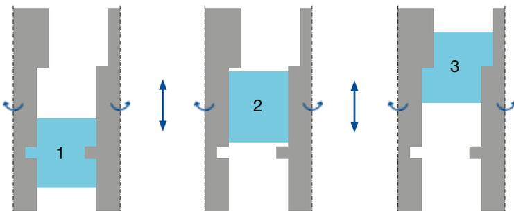
Different edge formation possible through vertical height adjustment of the combination tool.
