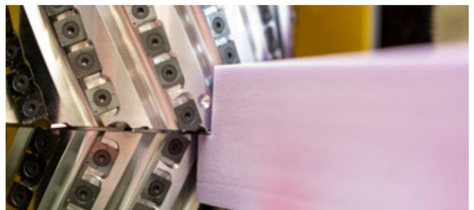
Examples for machining insulation materials – CentroFix (photo left side) for thickness calibration and HeliCut (photo right side) for lateral processing.
