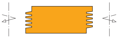
Profile 2 with staggered shoulder cutters
