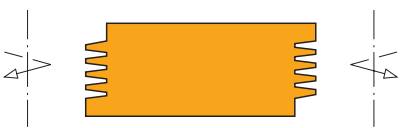
Profile 2 with staggered shoulder cutters
