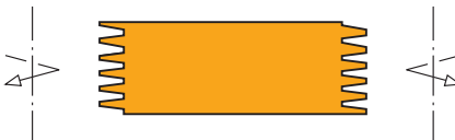
Profile 1 with continuous finger jointing
