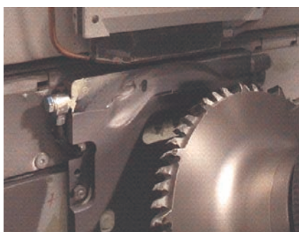
Problem: Machine wear through abrasive chips.
