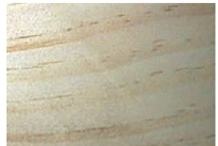
Finish planed surface after preplaning with RipTec.
