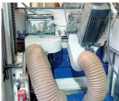
Problem: Machine wear through abrasive chips.
