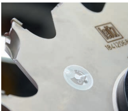
Tool with integrated NFC Chip
