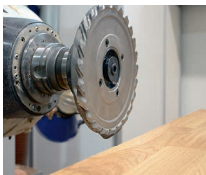
DFC® tool for directed chip beam. DFC®-system: Tool with adapted extraction hood. Most of the chips are collected and the wear is kept away from the machine.
