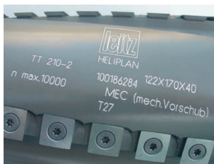
Labelling example of boring tools.
