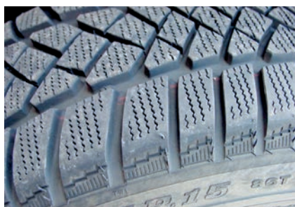
Tire profile with irregular pitch.
