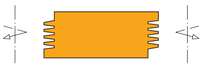
Profile 2 with staggered shoulder cutters
