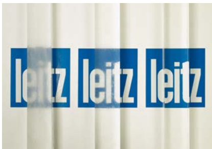
Gloss cut section on PMMA workpiece
