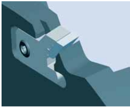
With advanced shear angle outside.
