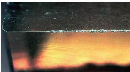
DM edge - monocrystalline synthetic diamond
