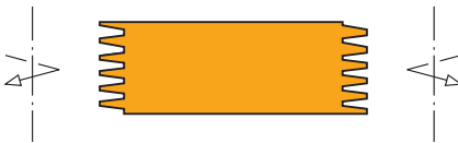
Profile 1 with continuous finger jointing
