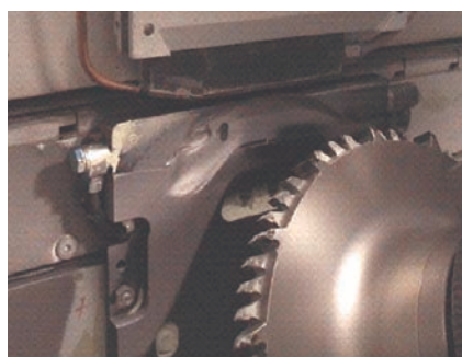
Problem: Machine wear through abrasive chips.
