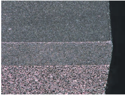
DP edge polycrystalline diamond layer (on top) sintered on to a tungsten carbide substrate (on bottom)
