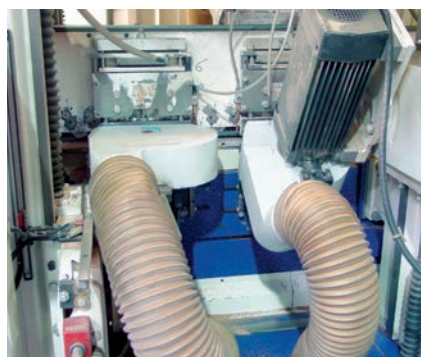
Problem: Machine wear through abrasive chips.
