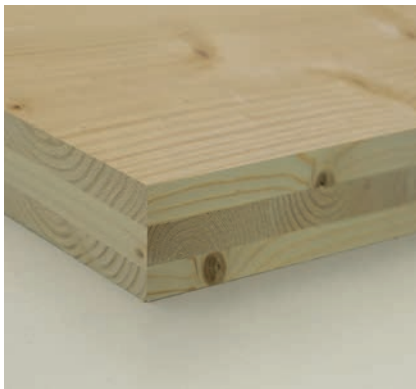
Cross laminated timber CLT
