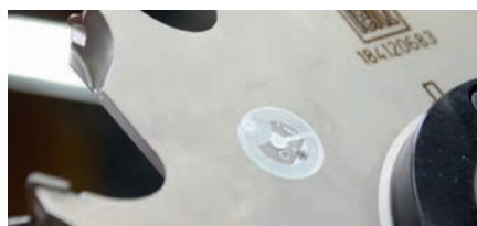
Tool with integrated data chip.
