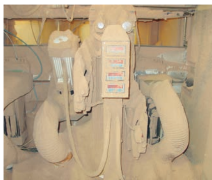
Laminate processing: Typical chip collection in the machine.
