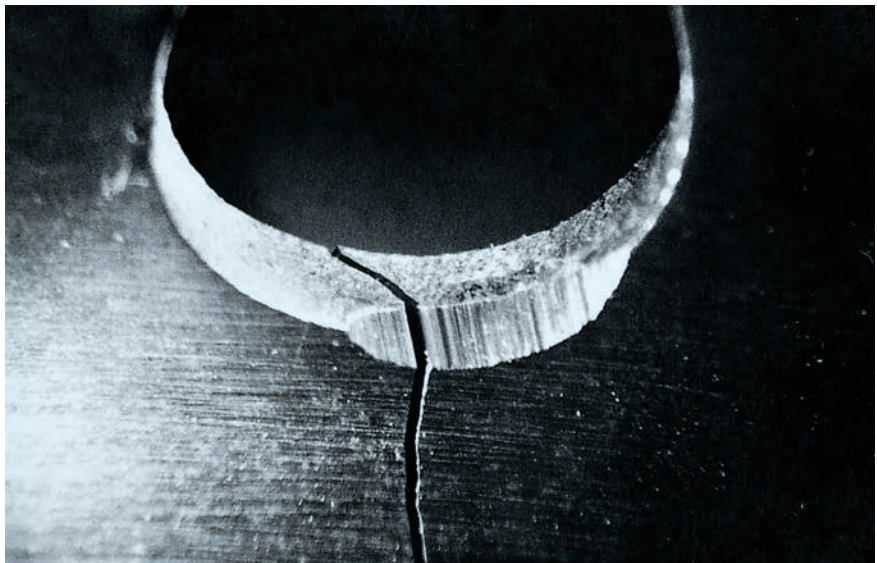
Fracture in the saw body.
