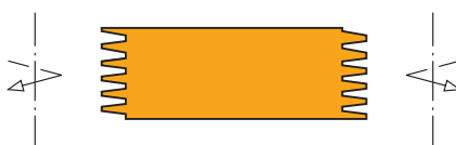
Profile 1 with continuous finger jointing
